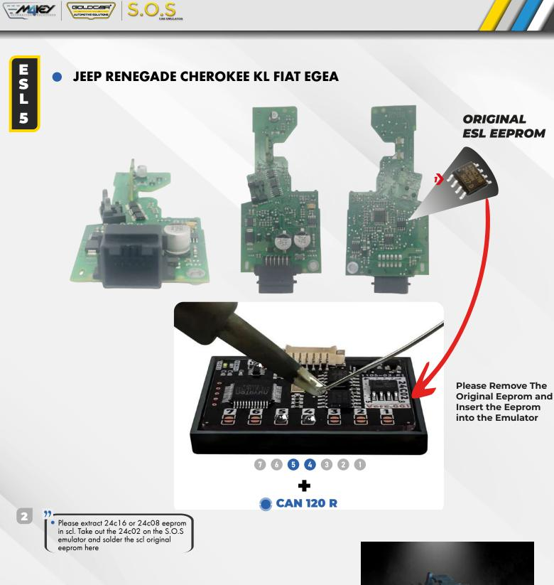
Connect the Emulator to the SCL plug according to the pictures on the right.
