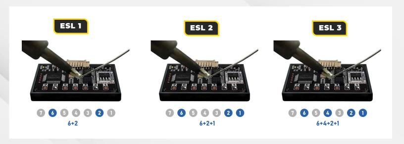
If the Emulator doesn't work, solder an additional jumper CAN 120R
